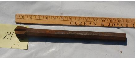
This is used to shape hot iron, or to possibly to size a hole. The blacksmith would hold the hot iron in place on the anvil and his helper would hit it with the flattening tool, driving it right through the hot steel.
